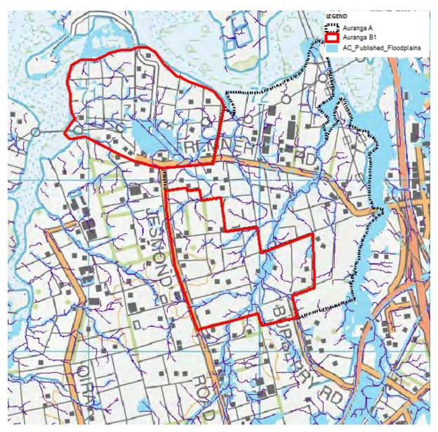
Figure 3-3: Existing 1% AEP floodplain (light blue) and overland flow paths (dark blue lines) for Auranga B1 (from Auckland Council Geomaps)
